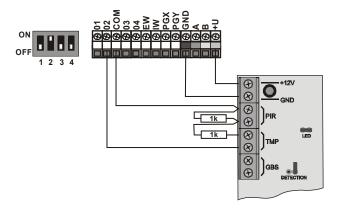
fig. 3 JS-20 Largo detector connection
