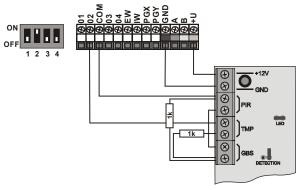
fig. 4 One-loop connection of JS-25 Combo
