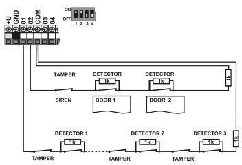
fig. 6 Connection of multiple detectors to the inputs
