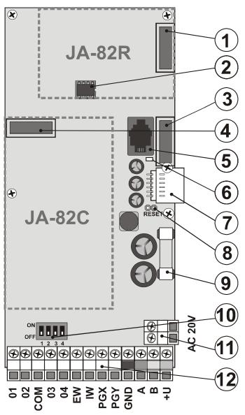
fig. 1 Control panel main board
