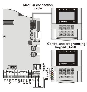
fig. 7 Wired keypad connection
