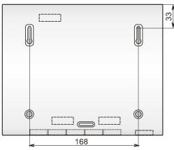
fig. 16 Control panel box dimensions
