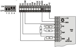
fig. 5 Two-loop connection of JS-25 Combo (01 GBS, 02 PIR)
