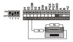
fig. 2 SA-200 magnetic detector connection
