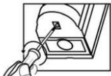
1. Remove the screw on the bottom (next to the tag reader)
