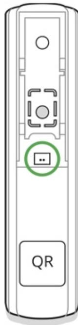
We recommend installing the wired detector at a distance no longer than 1 meter to DoorProtect Plus. Longer wire length increases the risk of its damage and reduces the quality of communication between the detectors.
