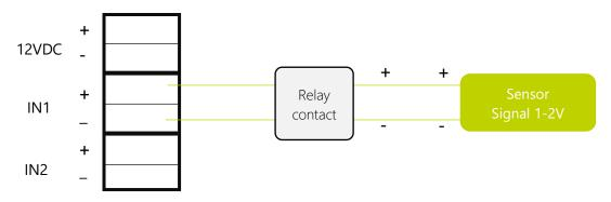
3. Alarm signal between 2V - 48V
