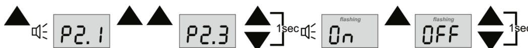
Figure 6. Example of setting the P2.3 parameter after activation of the thermometer and with the F2 operation mode selected
