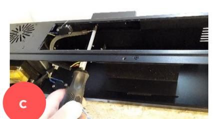
Fit, and ensure tight, 1x M6 set screw with washer in the 2 holes in the back of the Smoke Screen alongside each of the two mounting slots. Access to the fixing holes is through the fluid and heater block compartments.
