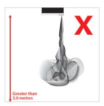
The optimum ceiling mounting height for the Smoke Screen is 2.5 metres above the floor over the area to be protected and using a straight nozzle. The maximum mounting-height above floor level is 3 metres and there should be no obstacle within 1 metre of the smoke output nozzle.
