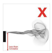
The optimum wall mounting position for the Smoke Screen is 2.5 metres above the floor facing the area to be protected and using an appropriate angle nozzle. The maximum mounting-height above floor level is 3 metres, the minimum is 1 metre and there should be no obstacle within 1 metre of the smoke output nozzle.
