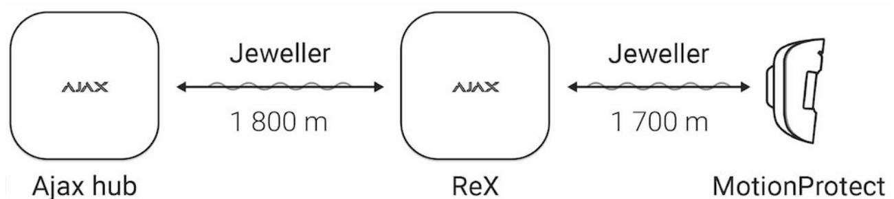
The communication range between ReX and the device is limited by the radio signal range of the device (indicated in the device specifications on the [website](#) and in the User Manual).
