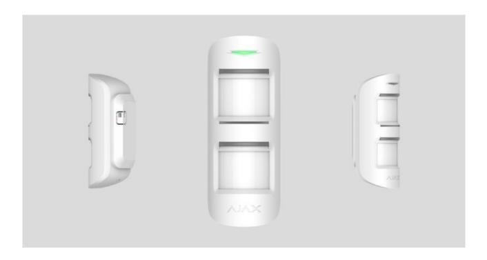
MotionProtect Outdoor is a wireless outdoor motion detector for the Ajax security system. The detector communicates with the hub via protected <a href="Jeweller">Jeweller</a> radio protocol at a distance up to 1,700 meters in the line of sight. MotionProtect Outdoor features protection against blocking the detector view (anti-masking system) and triggering by pets (pet immunity). The motion detection distance is adjustable: from 3 up to 15 meters.
