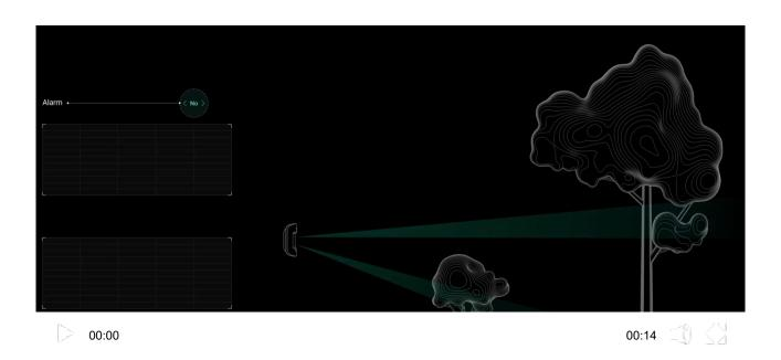
MotionCam Outdoor features two independent IR sensors, the signals of which are analyzed by a two-stage LISA algorithm. As soon as both IR sensors detect movement, LISA performs correlation and spectral analysis of the signals, which allows you to instantly distinguish between real threats and interference.
