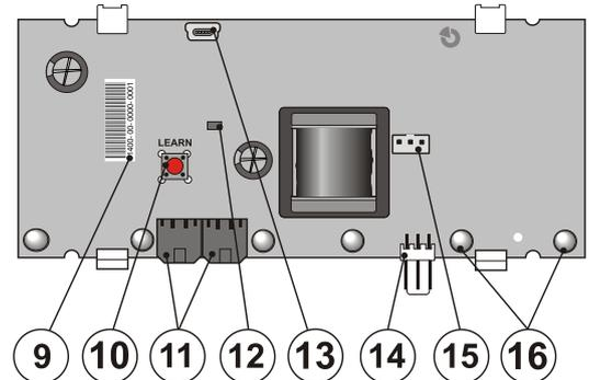
Figure 2: 9 – production code; 10 – LEARN (enrollment) button; 11 – battery connector; 12 – yellow fault indicator; 13 – mini USB connector; 14 – piezo siren connection (attention: high voltage); 15 – external antenna connector; 16 – high intensity red LED flashers
