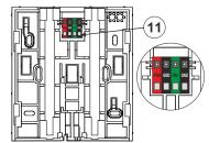
Figure 4: 11 – terminals of an external power supply and an external magnetic contact
