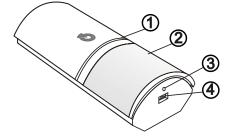
Figure 1: 1 – LED indicators, 2 – PIR lens, 3 – Hole for locking screw, 4 – Cover tab
