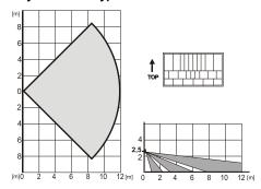
Figure 3. This detection characteristic is valid for standard PIR immunity.
