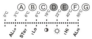
Figure 2: A – Low temperature, B – Temperature in Standby mode, C – Lower temperature limit pre-settable by user, D – Economical temperature, E - Comfort temperature, F - Upper temperature limit pre-settable by user, G - High temperature
