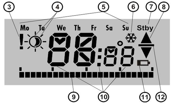
Figure 3: 3 – Internal settings entry by F-Link SW/ communication fault; 4 – Symbols of comfort ⊙ and economical ⊖ temperatures; 5 – Days of the week; 6 – heating activated when thermostat is blocked; 7 – Standby mode activated; 8 – Heating, flashing ▲ – thermostat blocked by open window for example; 9 – Axis of heating periods; 10 – Symbols for showing the temperature, time and text; 11 – Not used; 12 – Showing the pre-set / required temperature
