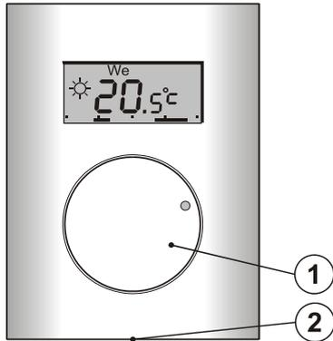
Figure 1: 1 – Knob combined with a button; 2 – Cover tab
