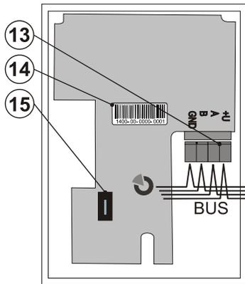
Figure 4: 13 – Terminals for BUS to be connected;
