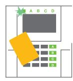
1. Authorize yourself using the keypad (enter a code or hold an RFID card or tag up to the reader). The system indicator button will start flashing green.
