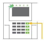
2. Press the function button to set a particular section. It is possible to set more sections subsequently. The delay between sections selection must not be longer than 2 seconds.
