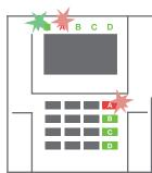
1. When you enter the building (triggering a detector with a "Delayed zone" reaction), the system starts indicating an entrance delay with a continuous tone, the system indicator and a function button, both flashing red, of the section in which the delayed entrance has been triggered.
