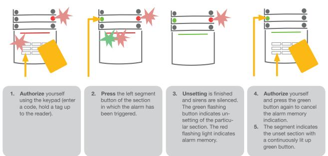
2.2.1.5 TERMINATING A TRIGGERED ALARM
