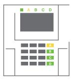
**3.** The command is executed and the function button turns permanently yellow to indicate a partially set section. To set the entire premises in which partial setting is enabled, hold down the button to set the control panel for 2 seconds or press it twice. After the button is pressed once it shows continuous yellow light, after it is pressed a second time it shows continuous red light.
