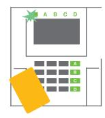
1. Authorize yourself using the keypad. Function buttons A, B, C, D will light up and the system indicator starts flashing green.
