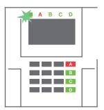
3. The command is executed and the keypad acoustically indicates the exit delay. The section is set now, only the detectors with a "Delayed Zone" reaction provide time to leave the guarded area during the Exit delay. The status indicator and a function button of the set section will turn red.
