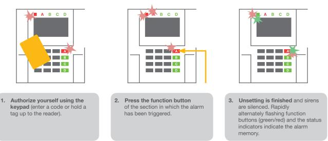
A triggered alarm in progress is indicated by the status indicator and the function button rapidly flashing red. You need to authorize yourself using the keypad in order to terminate the alarm. The section remains set, a rapidly flashing red function button indicates the alarm memory. Indication will continue flashing even after the system has been unset.
