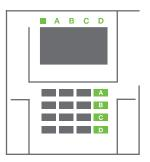
The command is executed. The function buttons and the system indicator turn green to indicate unset sections.
