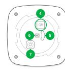
To switch on the siren, press and hold the On/off button for 3 seconds. The siren is switched off in the same manner. If the siren is not linked to the hub, it will automatically power down 6 seconds after activation.
