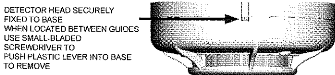
Figure 3: To Remove a Locked Sensor From the Base
