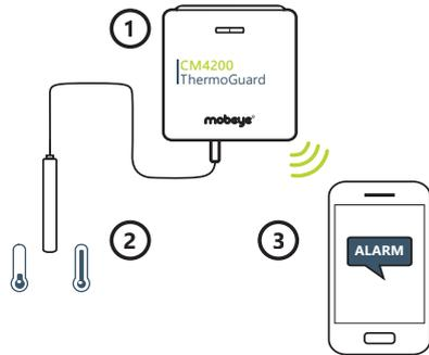
The Mobeye CM4200 continuously measures the temperature values. The alarm dialer immediately sends a notification if it gets too cold or too hot. In this way you have full control.
