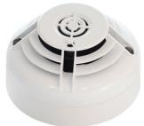
The sensing elements of the SMART3 are panel controllable so the sensitivity thresholds of each element can be changed by the panel offering the ability to customise the device for the changing use of the area it is protecting. The detector has built in short circuit isolation and two integral tri-colour LEDs that provide 360° local visual indication of the device status. The LEDs are programmable with static or blinking red, amber and green status indications available.
