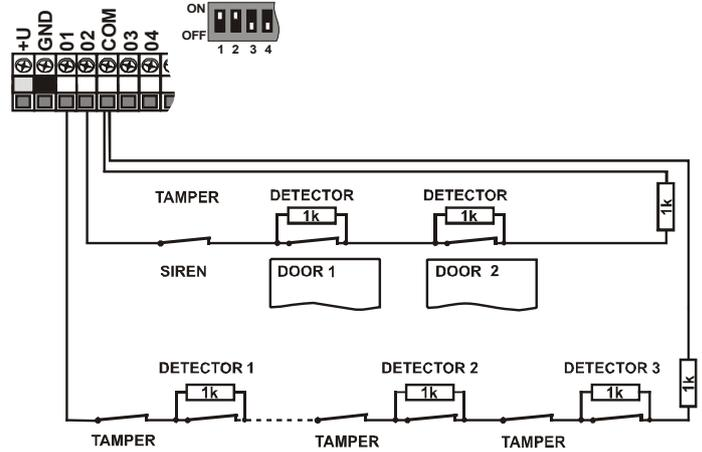
fig. 6 Connection of multiple detectors to the inputs
