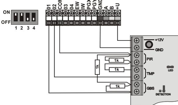
fig. 5 Two-loop connection of JS-25 Combo (01 GBS, 02 PIR)
