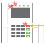
2. Press the function button of the section in which the alarm has been triggered.
