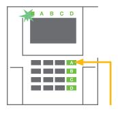
Press the function button to set a particular section.
