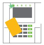
1. Authorize yourself using the keypad (enter a code or hold an RFID card or tag up to the reader). The system indicator button will start flashing green.
