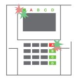
Unsetting is finished and sirens are silenced. Rapidly alternately flashing function buttons (green/ red) and the status indicators indicate the alarm memory.
