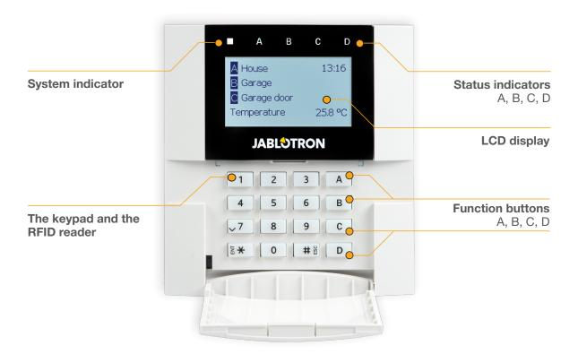
Statuses of individual sections are indicated by status indicators A, B, C, D above the LCD display and by the functions buttons. The control panel can be operated directly (setting or unsetting the alarm and other automation functions) using function buttons on the keypad. The function buttons and the status indicators A, B, C, D are colourfully backlit in order to clearly indicate the section status.
