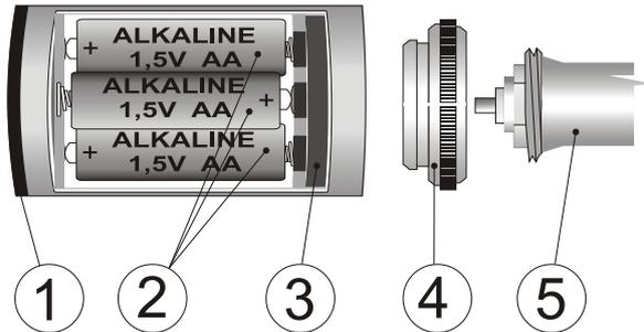
Fig. 1: 1 – indicator; 2 – batteries; 3 – safety ring; 4 – adapter; 5 – radiator valve
