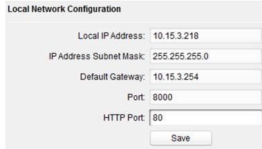
The screenshot shows a web form titled "Local Network Configuration". It contains five input fields and a "Save" button. The fields are: "Local IP Address" with the value "10.15.3.218", "IP Address Subnet Mask" with the value "255.255.255.0", "Default Gateway" with the value "10.15.3.254", "Port" with the value "8000", and "HTTP Port" with the value "80".
