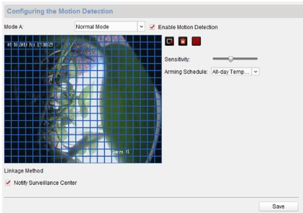
**Figure 1-21 Motion Detection**
