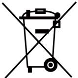
2006/66/EC (battery directive): This product contains a battery that cannot be disposed of as unsorted municipal waste in the European Union. See the product documentation for specific battery information. The battery is marked with this symbol, which may include lettering to indicate cadmium (Cd), lead (Pb), or mercury (Hg). For proper recycling, return the battery to your supplier or to a designated collection point. For more information see: [www.recyclethis.info](http://www.recyclethis.info)
