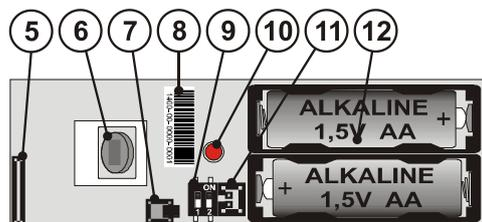
Figure 2: 5 – Antenna; 6 – PIR sensor; 7 – Tamper contact; 8 – Production code; 9 – Setting DIP switches; 10 – Red LED indicator; 11 – The JA-191PL external tamper connector; 12 – Battery holder
